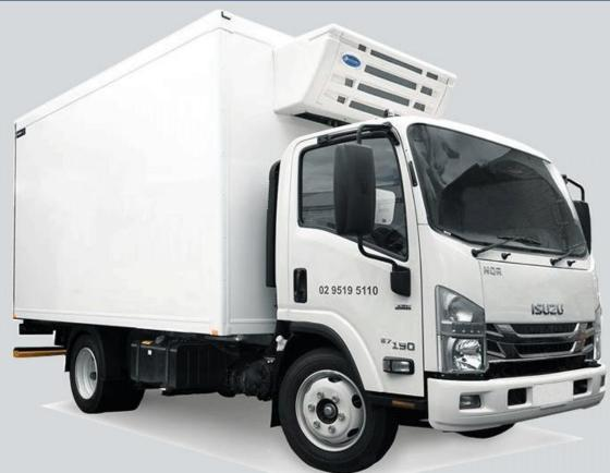
Guchen Thermo integrated standby units are with the scroll electric compressor inside the condenser units, that can be plug into external AC power supply when truck engine stops. *Saving Fuel/ Saving Money/riendly Eco-f.* The compact and integrated structure are *light-weight, low noise, low failure rate, easy for installation and maintenance!*
